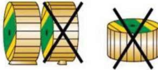
Do Not Lay Drums Flat On Their Sides, Use Proper Wedges To Prevent Drums Rolling
